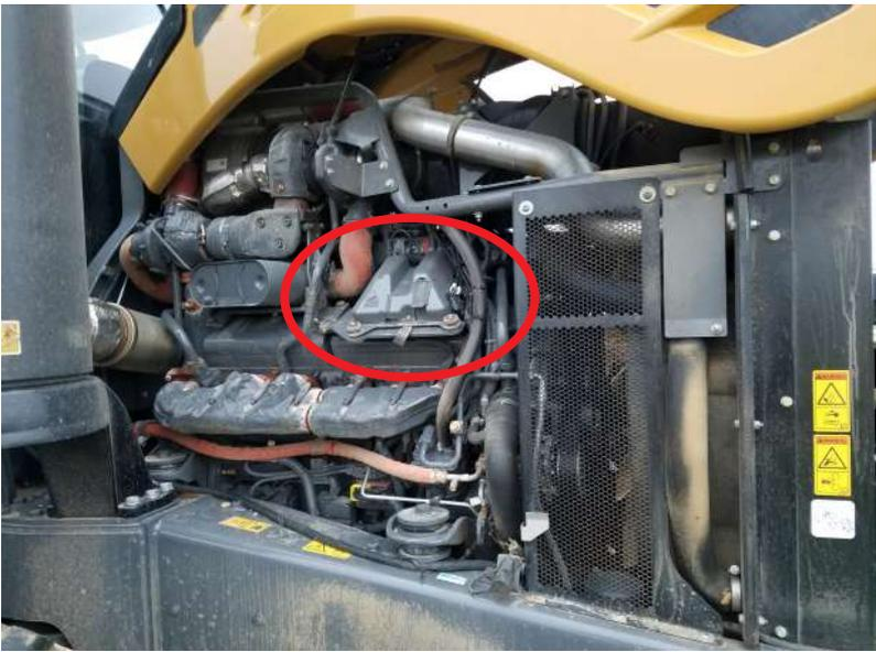
You will be working on both sides of the tractor as it works off of two ECM controllers. Picture above is the “passenger” side and the ECM is in plan view. You will have to remove the plastic cover to access the ECM harness plug.
